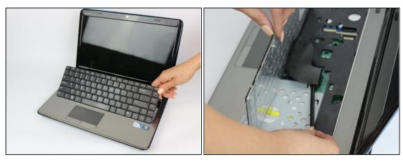
• Carefully tip the keyboard upwards and pull it slightly away from the body of the laptop.
