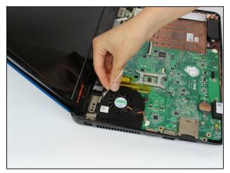
• Remove the fan from the device.
