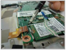
To unscrew the mainboard use the Phillips #0 Screwdriver to remove two types of screws. Three
