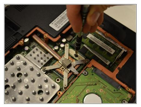
Using the traditional 2.5mm screwdriver, rotate the locking tab counterclockwise to unlock the graphics card.
