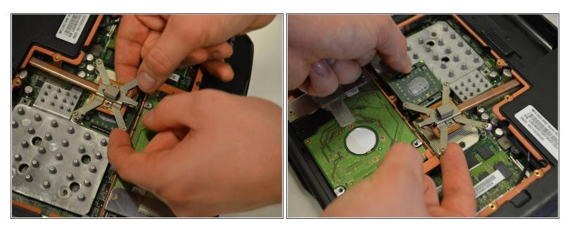
• Lift up the heat sink line and remove the graphics card.
