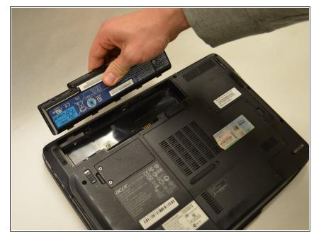
Grasp the inside edge of the battery and lift to fully detach the battery from the computer.
