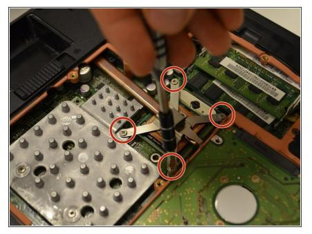
Unscrew the four 0.5mm Phillips #1 screws located on the heat sink in numerical order, as labeled on the device.
