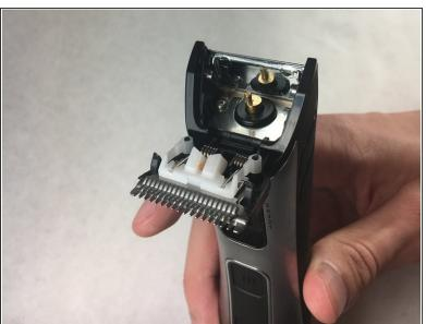
Place thumb behind trimming blade and push up to open.
