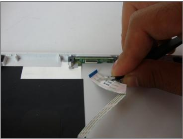
• Use the <u>tweezers</u> to gently remove the white pogo board ribbon from the hinge connector.
