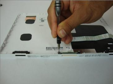
Use the Phillips #0 screwdriver to unscrew 2 screws 2.82 mm head 3.5 mm length from the hinge connector
