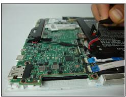
• Carefully disconnect the battery cable from its connector on the mainboard.
