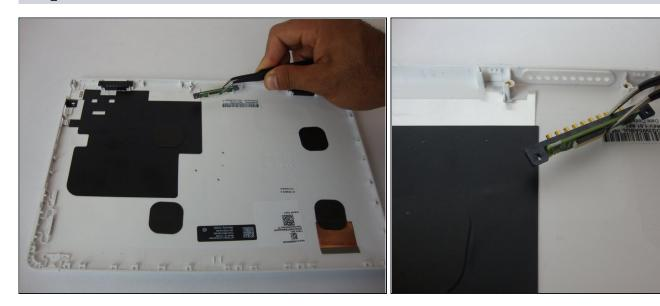
• Gently remove the hinge connector from the display panel.
