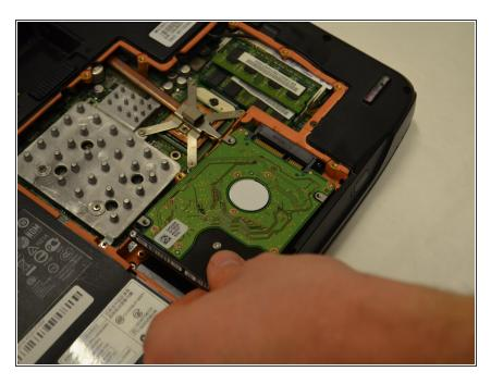
Remove the hard drive from the device.
