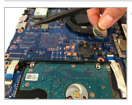
Fully remove the CMOS battery from the motherboard. To reassemble your device, follow these instructions in reverse order.
