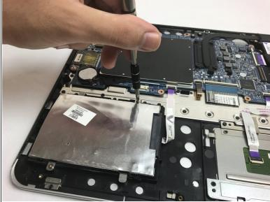
Use a JIS J1 bit to remove the two 4.6 mm screws.
