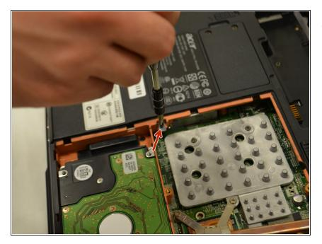
Remove the .5mm Phillips #1 black screw located on the left side of the panel opening.
