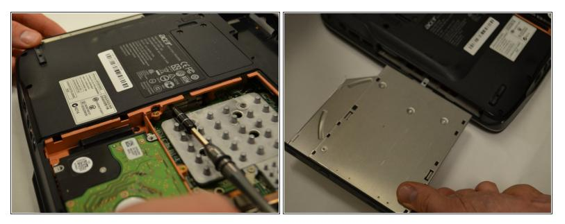
• Using the screwdriver, push the CD drive out of the laptop through the panel exposure.
