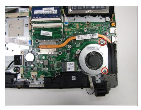
Unscrew the two 0.5 mm screws using a <u>Phillips #00 screwdriver</u>.
