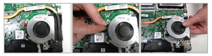
• The fan is connected to the motherboard by a cable. To disconnect the fan, gently push in the sides of the connecter to lift the base of the cable out of the port.
