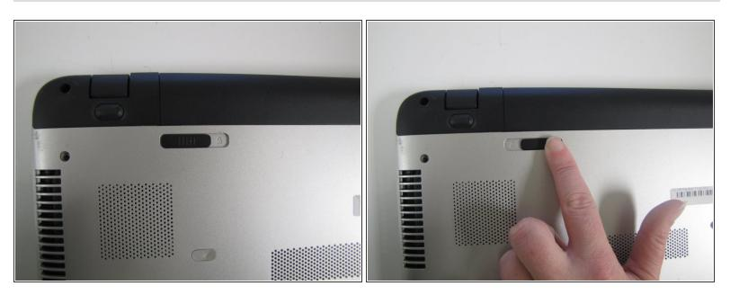
In the upper left hand corner, slide the bar with the lock icon to the right. This will unlock the battery.
