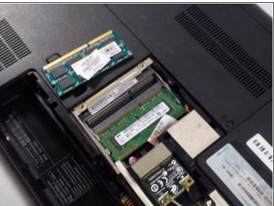
If you need to remove memory before installing the new memory, release the memory using a small wooden tool, or fingernail, to spread the clips holding the memory.
