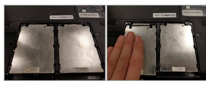
Firmly press with your hand on the silver surface and pull back, dislodging the hard drive from its port.
