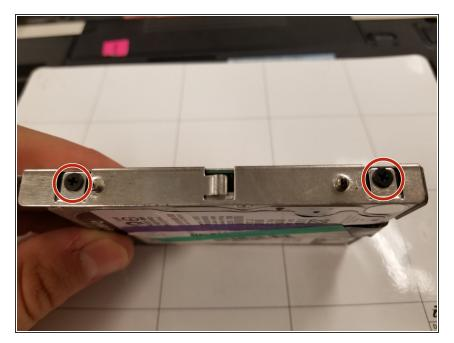
Remove the four 1.2mm screws attaching the case to the hard drive.
