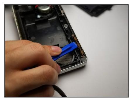
The buttons will be on the side of the device, use the plastic opening tool to remove it from its actual place no need to use any screwdrivers.
