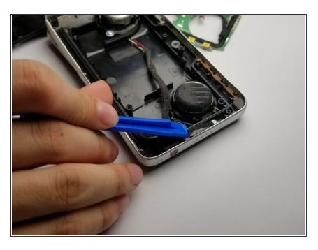
Use the plastic opening tool to remove the indicator lights and replace them by new ones.
