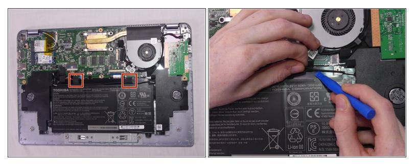
• Remove the tape holding the speaker wire to the battery on both sides using a small opening tool.
