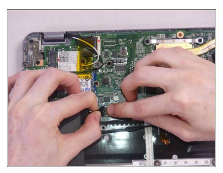
Gently remove wire from the motherboard by pulling it out of the connector socket.
