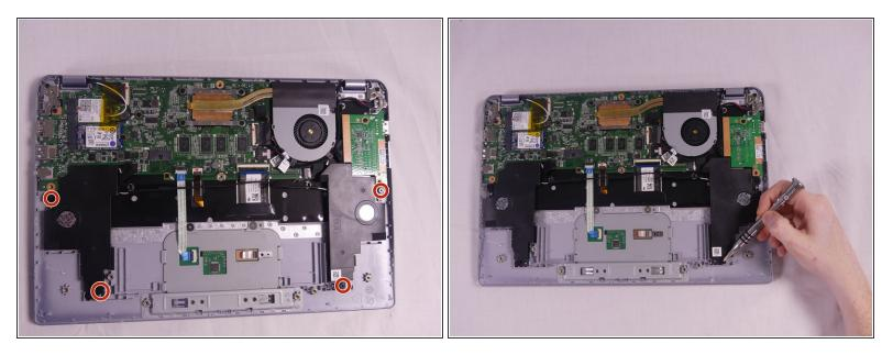
Remove the 4 Phillip 6.3 mm screws from both the right and left speakers using Phillips 1 screwdriver.
