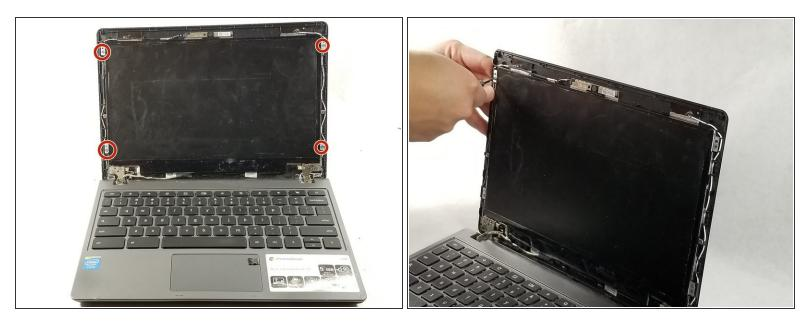
• Remove the four 3.4 mm screws by using the Phillips #0 screwdriver.
