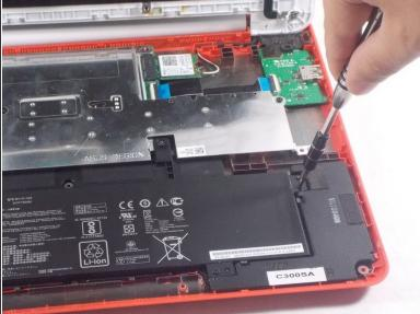
Remove the six 5.6mm Phillips #0 screws around the battery.
