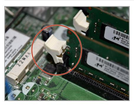
Push out securing clips and remove used RAM sticks.
