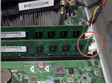
Clear aside internal wires and locate RAM sticks secured by clips.
