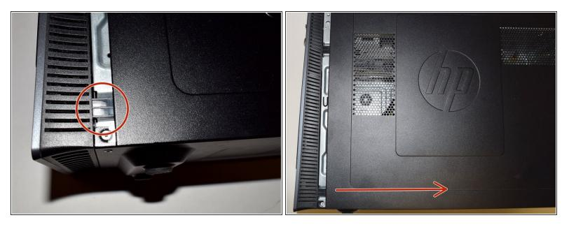
Safely place the computer down on its side and slide the panel off the case.
