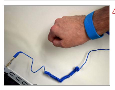
⚠ Due to the potential of painful electric shocks, an anti-static wristband clipped to an unpainted piece of metal on the computer case is highly suggested.
