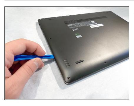
Slide an opening tool between the base and back cover and work your way around the entire device to release the back cover.
