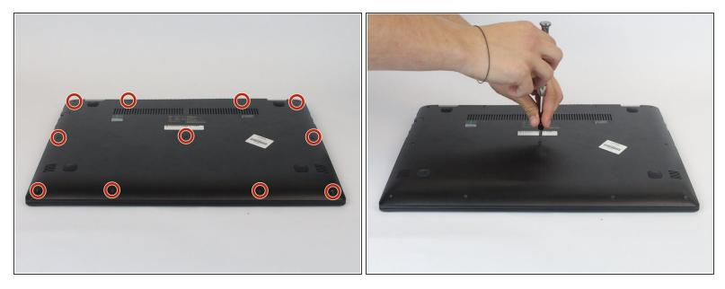
• Using the Phillips #0 screwdriver, remove the (11) eleven 5.4 mm screws from the back panel.
