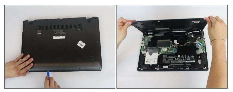
Using a plastic opening tool, pull out the back panel from the laptop.
