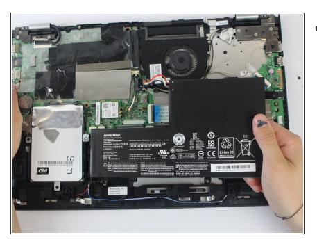
Pull the battery outward and remove it from the rest of the laptop.
