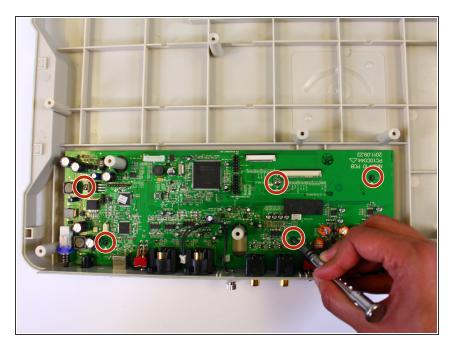
Loosen and remove the five 12mm screws from the circuit board using a Phillips #2 screwdriver.
