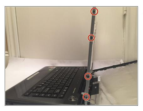
Remove the eight 6.5 mm screws on the left and right sides of the screen using the Phillip's #0 screwdriver.
