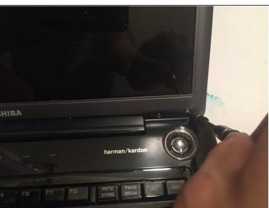
Remove the six 5.8 mm screws using the Phillip's #0 screwdriver.
