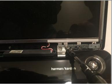
Remove the four 5.8 mm screws using the Phillip's #0 screwdriver.
