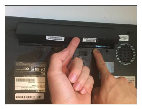
Carefully remove the battery from the laptop.
