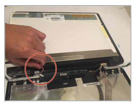
Remove cold cathode fluorescent light bulb connector.
