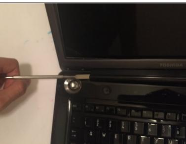
Pry out the bottom left and right locking pieces of the plastic housing with the metal spudger.
