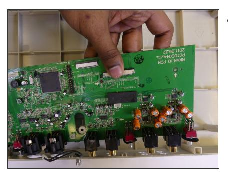
Carefully remove the circuit board from its housing.
