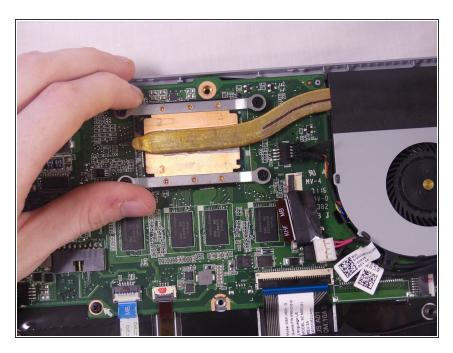
Lift up on the metal plate that hold the screws to start removing the fan.
