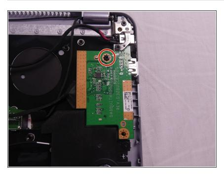
Remove the Phillips 3.7 mm screw using a Phillips #1 screwdriver.
