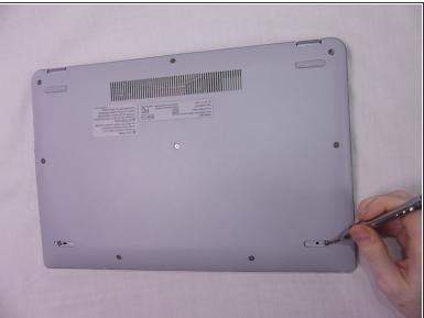
Remove the 10 7.1 mm screws using Phillips #1 screwdriver.
