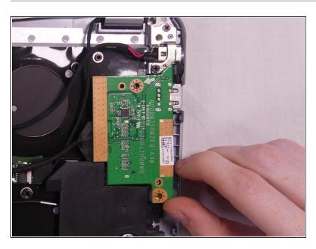
Gently remove the WiFi PCB by pulling upward.
