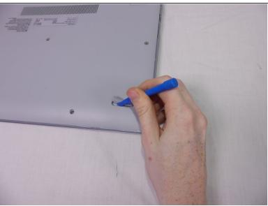
Remove the 2 rubber foot pads from the bottom (opposite the hinge) with the small Plastic Opening tool.
