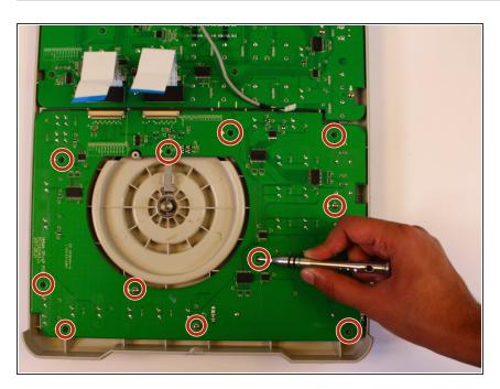
Loosen and remove the 11 12mm screws from the circuit board using Phillips #2 screwdriver.
