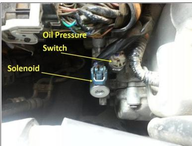
Use a size 24 socket with extension bar to remove the Oil Pressure Switch.
