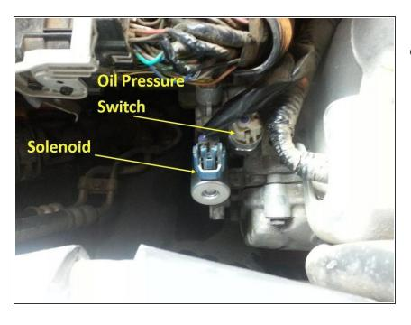
Disconnect the electrical plugs from the solenoid and oil pressure switch.
