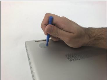
• Use the plastic opening tool to remove the gray rubber pads on the bottom of the laptop. For our device we only needed to remove the two at the top.
