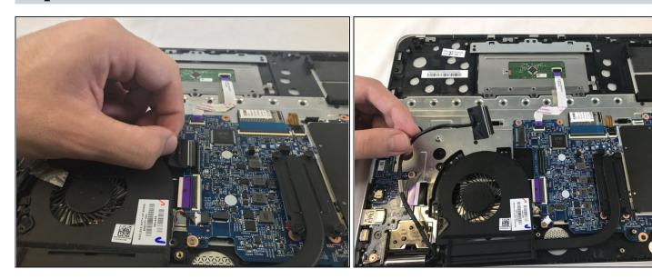
• Use your fingers to lightly pull the cable and disconnect it from the motherboard.
