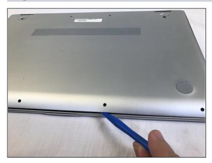
Use a plastic opening tool to pry open the case. Go slowly around the edge. You will hear popping noises, such are due to popping open the small joints that keep the cover attached.
