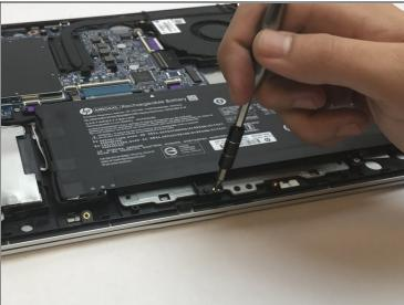
Use a JIS #1 screwdriver to remove the six 4.7 mm screws.
