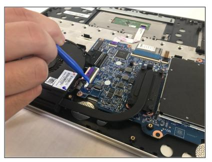
Use the plastic opening tool to disconnect the power cable from the fan.
