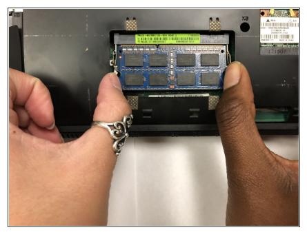
• Push the silver retaining brackets outwards to free the RAM stick(s).
