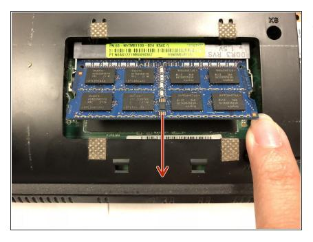
• Pull the RAM outwards after the RAM is lifted to remove the RAM.
