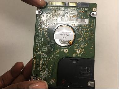
The hard drive should slide out of the laptop. However, if not, use a spudger to pry the hard drive out of the laptop.
