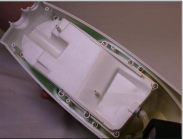
• Start by gently moving the midframe from the top portion of the panel to expose the bottom portion of the mop's water tank / bladder.
