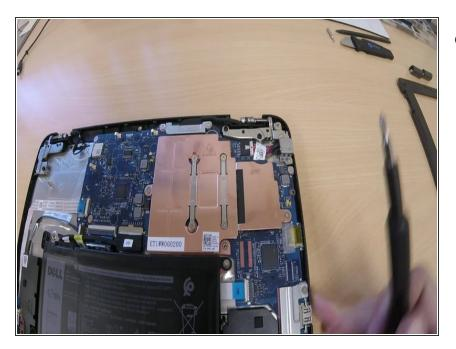
Using your phillips #0 screwdriver, remove the the 2 screws from the right metal hinge and the 3 screws from the left metal hinge.
