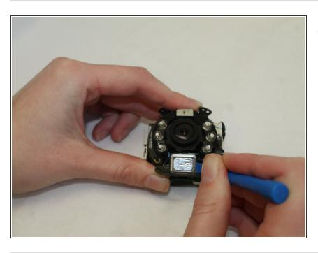
Remove the speaker using a plastic opening tool. The battery is attached with glue, so use gentle prying motions to remove speaker.
