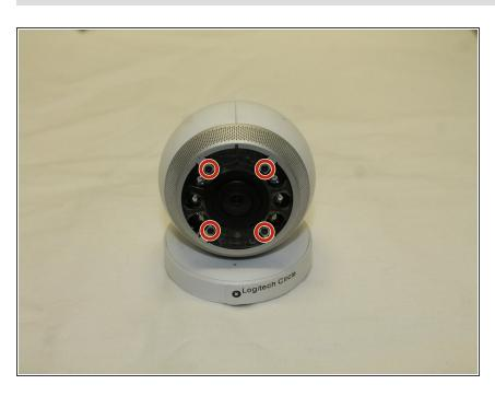
Remove the four 3mm Phillips #0 screws that hold down the first ring.
