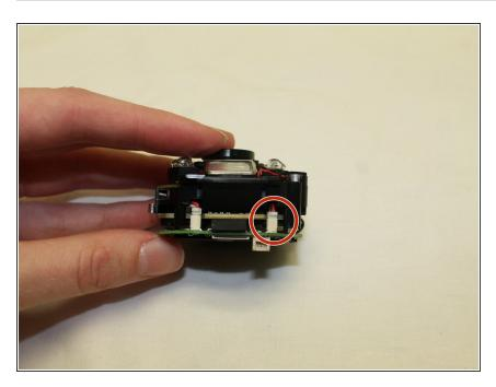
Locate the speaker attachment, and carefully remove the speaker plug from the lens.
