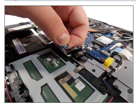
Pull tab until it disconnects from the trackpad. Be gentle you do not want to damage any part of the tab.
