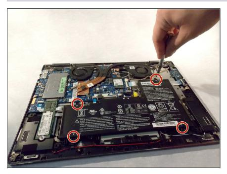
Remove the four 3.5 mm screws around the battery using the Phillips 00 screwdriver.
