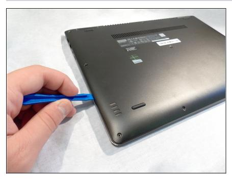
• Slide opening tool between the base and back cover.
