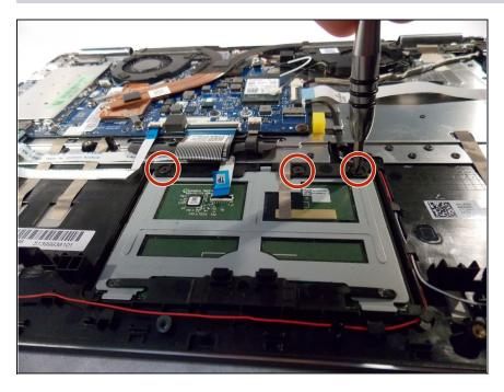
• Use the JIS 1 screwdriver bit to unscrew the 3 screws.
