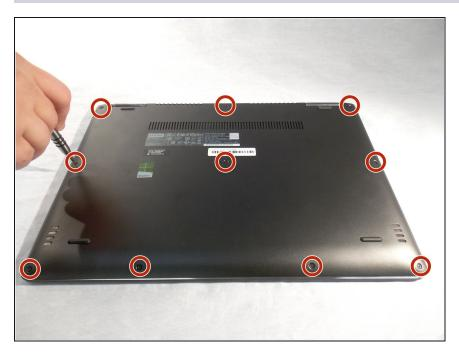
Remove the ten 3.3 mm screws from the base cover using the T5 Torx screwdriver.
