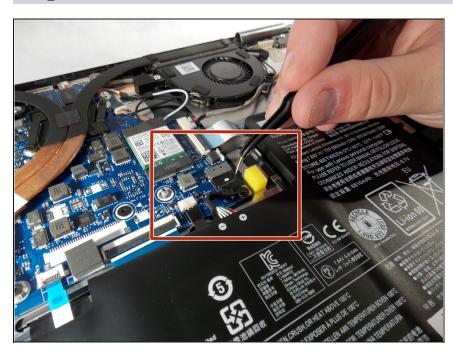
Disconnect the battery from the motherboard.
