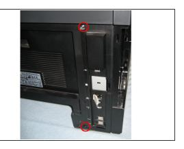
Loosen and remove front screws (1x top, 1x bottom) and rear (1x top, 1x bottom) with Phillips screwdriver.
