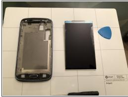
Remove the display with thin tools, using heat to detach the fixing adhesive
