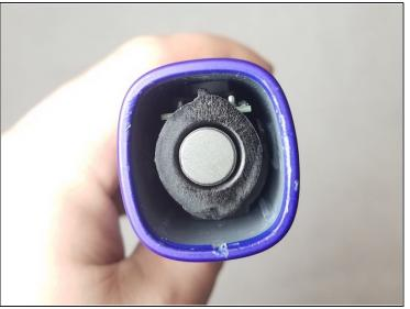
Use a nylon spudger to pry the chrome cap at the bottom off.
