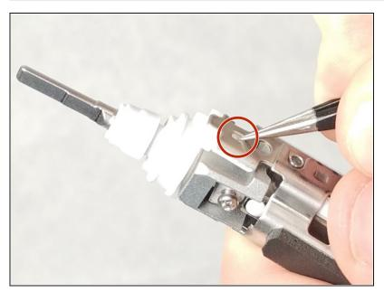
Use fine tip <u>tweezers</u> to push the white plastic tabs in to release the head from the innards.
