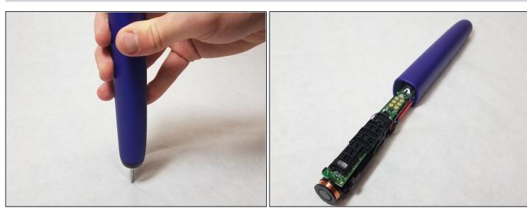
• Put the metal head on a solid surface with handle perpendicular to the surface. Firmly, yet gently, push down until the internals start to slide out.
