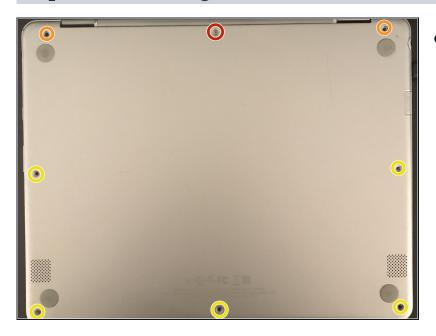
NOTICE: YOU MUST RE-INSERT THE BACK COVER THIS WAY IN ORDER TO KEEP THE PANEL FROM BULGING! Slide the cover into the back (hinge side first), make sure to slide in then push down on top to make sure cover is secured. Once secured, insert top middle screw first (red), then insert other top screws (orange), then the other screws (yellow).
