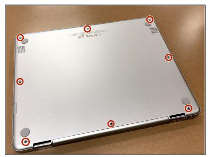
This step is very easy, use a PHILIPS#0 to remove the 8 screws on the back panel (flip computer upside down). There are no screws under the feet.
