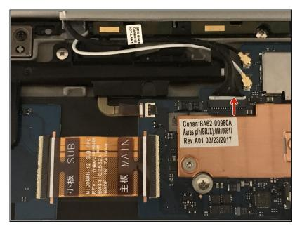
In the top left corner (with the battery at the bottom) where the arrow is pointing, pull the cable out of the socket.
