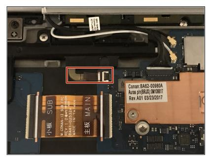
Remove the cable marked in this image by pulling on the pull tab. This will disable the s pen but will not physically remove it from the computer.
