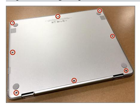
Remove the 8 PHILIPS#0 screws
