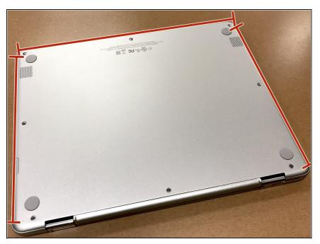
• Stick a <u>plastic card</u> (or fingernail) into the gap between panel and the body. Then lift the panel up (long side with speakers closest).
