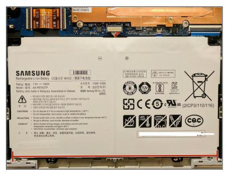
Lift battery from bottom side first (marked with red line)
