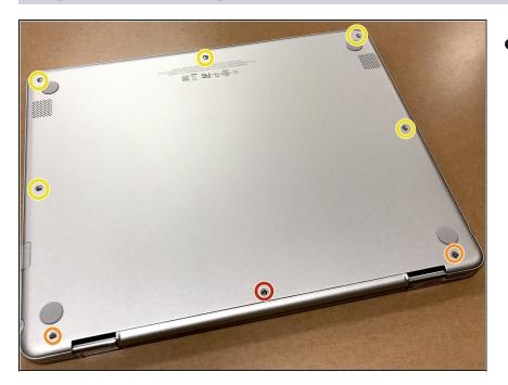
Insert the hinge-side middle screw (must be done first otherwise casing may bulge) and insert rest of panel. On the hinge side, press down on the sides (if there is bulging) until you hear it snap. Insert the two other hinge-side screws (marked with orange on image). After that, insert the other 5 screws (yellow).
