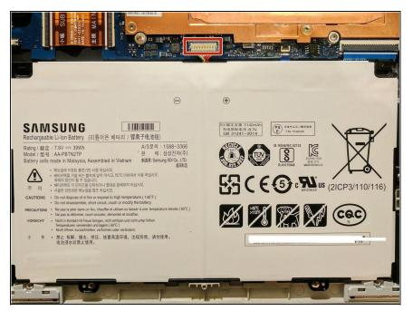
Insert the battery and push the plug into the socket downward.
