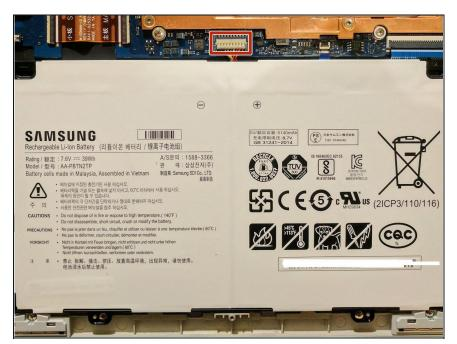
Detach battery cable grabbing the side and pulling the cable upward.
