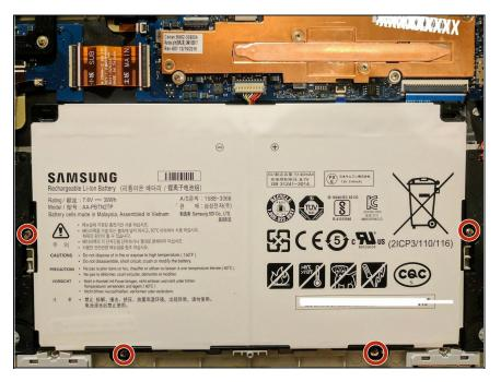
Re-insert the screws in the holes circled red (on this image), which is where you removed them previously.
