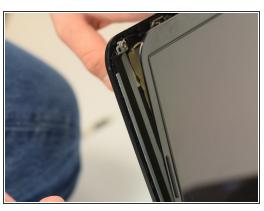
Using the pry tool, begin to separate the touchscreen from the plastic backing.
