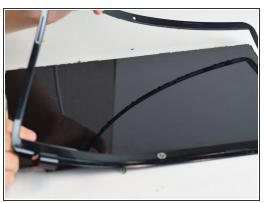
Using the sharp end of the pry tool, separate the plastic from the screen.
