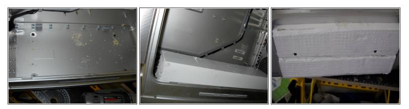
Drill 4 holes through the bottom of the case and put wood underneath the case and screw the wood pieces to the bottom of the mailbox. Put a piece of wood under the mailbox to have something to screw it to. You may have to drill more holes to screw the boards together with long screws.
