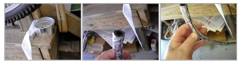
• Take a rubber fuel line and wrap it in silver hvac tape and slit the hose down the middle to make a seal to fill in the gaps between the mailbox. The silver tape is optional.
