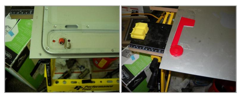
Insert an S hook and use pliers to close the S hook around the plastic connector to hold the flag on.
