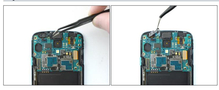
• Using a pair of precision <u>tweezers</u>, remove the black camera backing.
