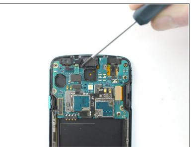
• Using the Phillips #00 screwdriver, remove the single 0.3mm screw securing the black cover over the camera sensor.
