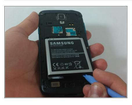
Insert a plastic opening tool, or your finger, into the notch of the battery compartment and lift the battery upward to remove it.
