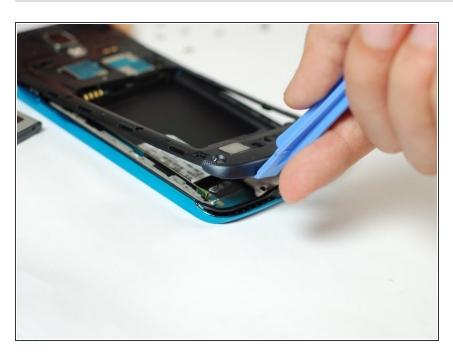
Use the plastic opening tool to pry around the entire edge of the midframe now to release it from the front case.
