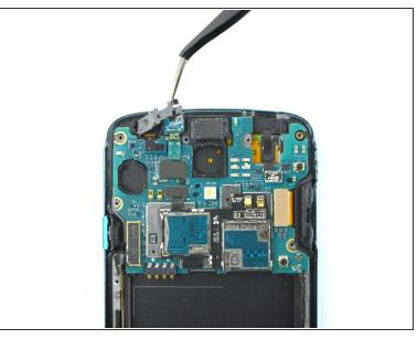
Using a pair of precision tweezers, remove the black camera backing.
