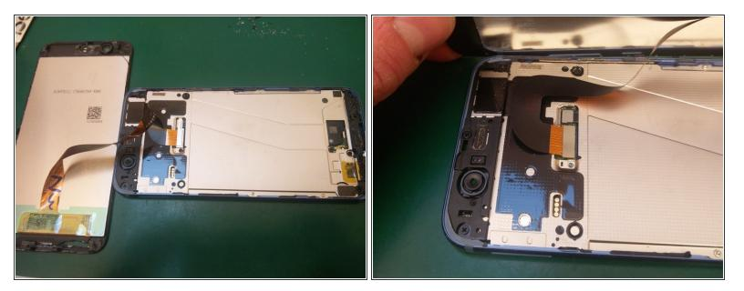
Now the display can be placed next to the device. Make sure that there are no excessive tensile forces or stresses on the connecting cable. Remove the Philips screw that holds the cover in place.
