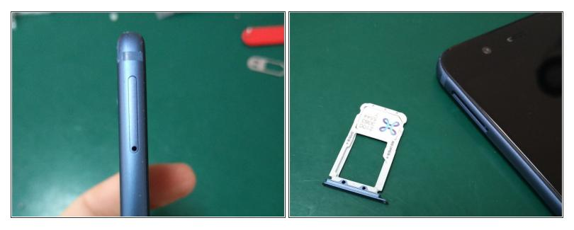
• To begin with, the sim tray is best removed. With this model and to do this repair it is not really necessary but in any case a good habit to start with.
