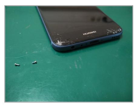
Remove the 2 screws at the bottom that hold the screen module in place.
