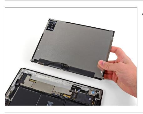
Remove the LCD assembly from the rear panel assembly.
