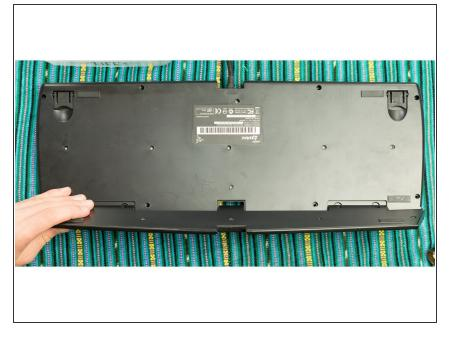
Lift the handrest plate and pull it free, away from the rest of the unit.
