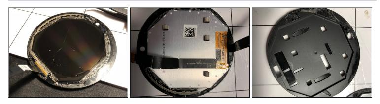
• Display module is round and glued to the cover glass
