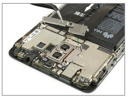
• Remove the cable bracket.
