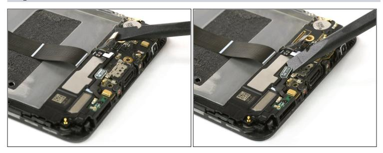
• Use a spudger to disconnect the loudspeaker and the charging port flex cable from the daughterboard.
