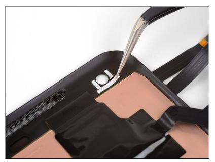
Peel the white backing off of all three adhesive strips.
