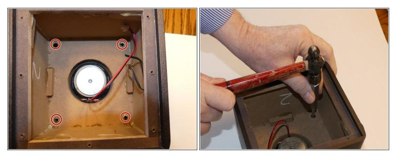
• Use a tap hammer and a punch to release the 4 posts that hold the front panel in place.
