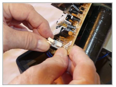
Remove the snap cable that connects the speaker to the circuit board.
