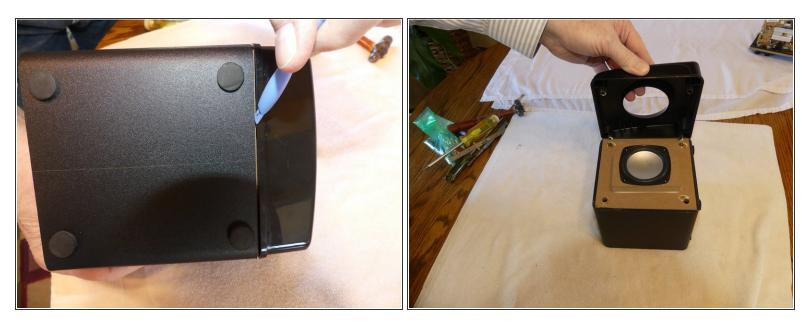
• Use a plastic opening tool or spudger to pry off the front panel.
