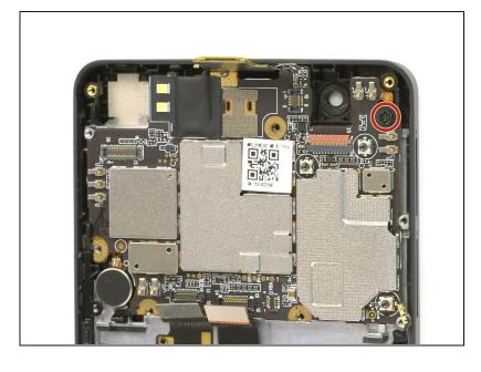
Take out the 4mm Phillips #00 screw, holding the mainboard to the frame.
