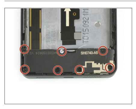
Take out the seven 4mm Phillips #00 screws, holding the loud speaker unit to the mid frame of the phone.
